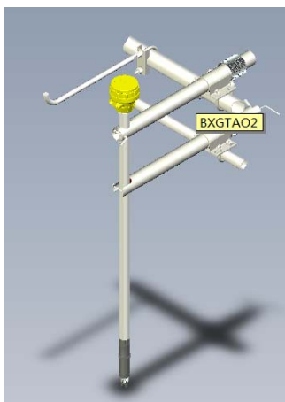
pH/ORP Scaffolding installation(P16)
